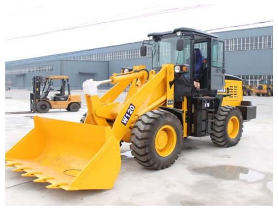
W120 mini wheel loader adopts torque converter and counter-shaft transmission gearbox-Komatsu technology, which can ensure higher reliability and easier maintenance. Fully hydraulic steering system and power shift transmission are employed in this machine. Therefore, the operation is easier the users. Bucket can be leveled automatically and there are many optimized working device that can be available easily. Therefore, the productivity of this kind of machine is higher.
